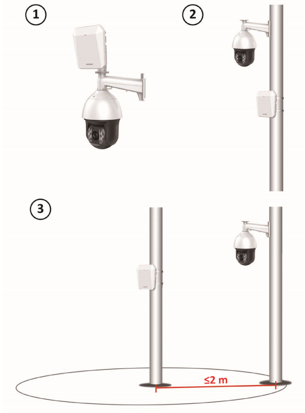
Figure 5-5 Installation Scene for One Point Calibration
