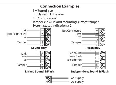
System status indication. (Permanently illuminates LED's at lower intensity.)
